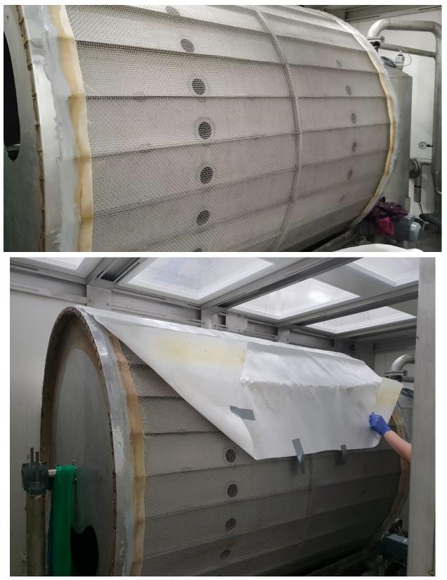
Figure 8: Pictures of the drum without and the cloth and during installation
