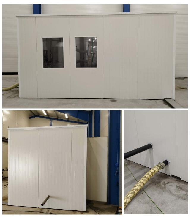
Figure 7: Outside views of the house – from top to bottom, left to right, side of the house / entrance door and screw conveyor / sludge inlet and filtrate outlet
