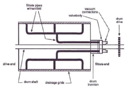
Figure 2: Schematic representation of the inside of the drum
